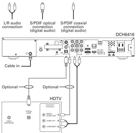
Note: Only (1) HDTV video connection needs to be made to an HDTV.
