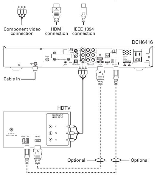
Note: Only (1) HDTV video connection needs to be made to an HDTV.
