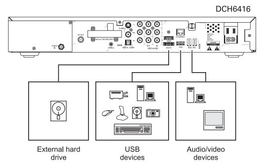
Do not attempt to connect data devices without contacting your service provider. Advanced data features require the proper application and network infrastructure to operate.
